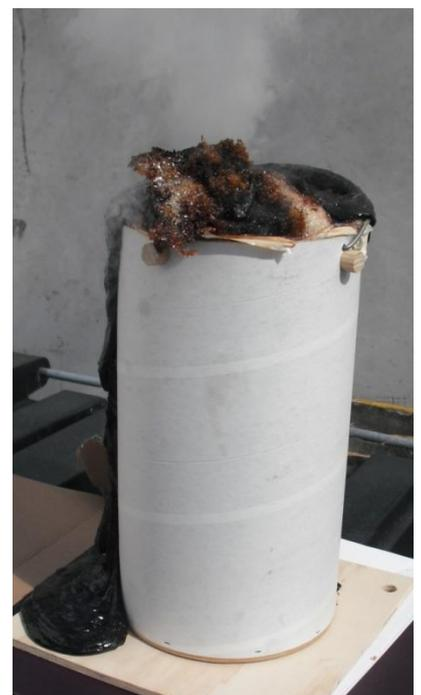
Let's look at our simplified infusion set-up again – this time with the resin catchpot in danger of overflowing.
